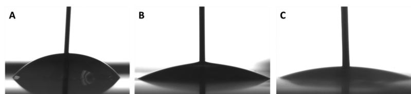
Figure 6. Receding contact angle measurements on (A) flat, (B) nanotube, and (C) annealed coating. Texturing of the surface leads to hydrophilic behavior, whereas the flat coating of the same alloy material shows hydrophobic-like behavior.
